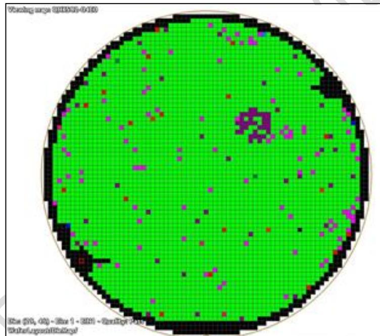
Fig. 1. Substrate mapping on front-end wafer testing
