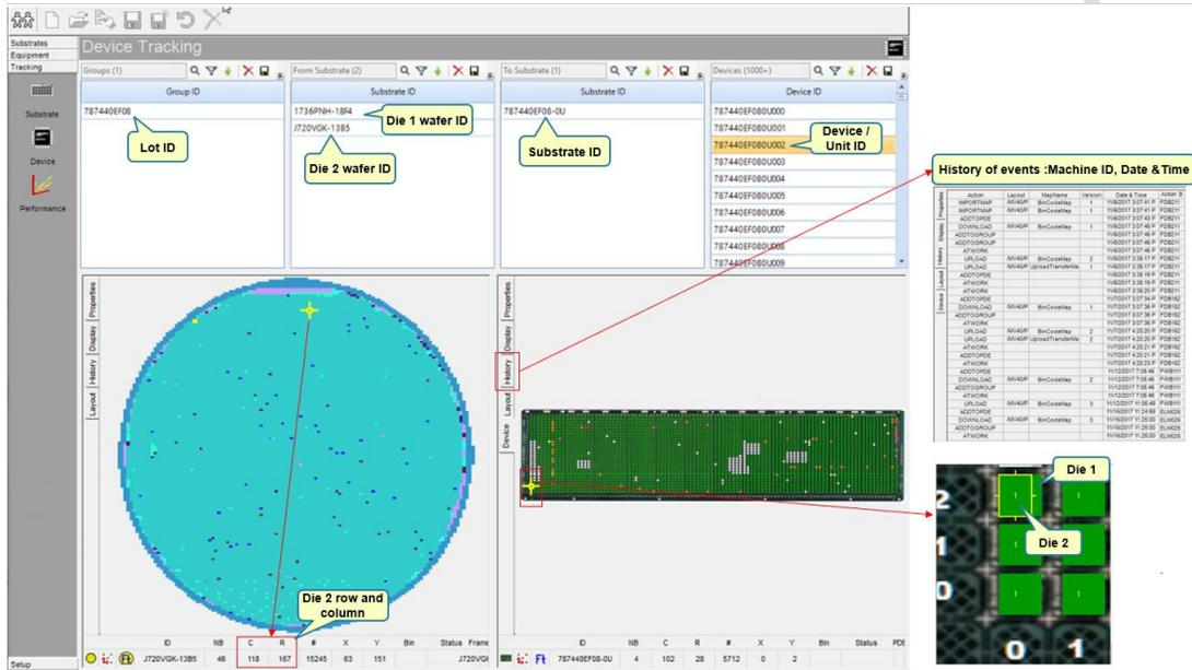
**Fig. 3. Electronic strip mapping with Single Device Tracking**
