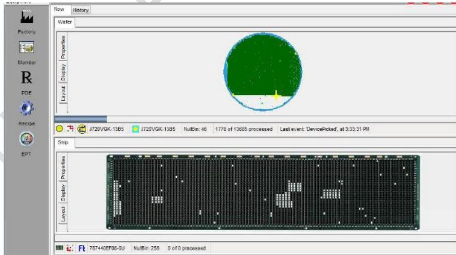
**Fig. 5. Completed strip at die attach showing good and bad units**
